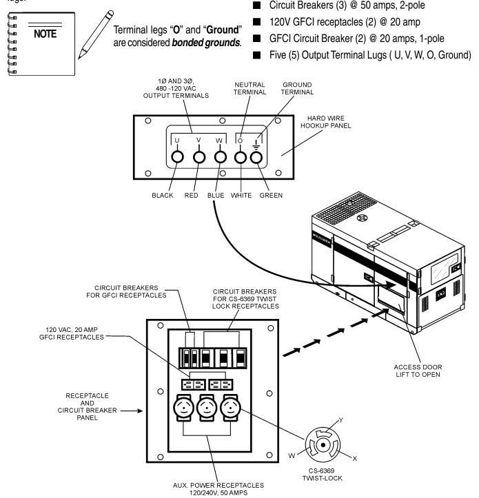
Figure 8. Output Terminal Panel
